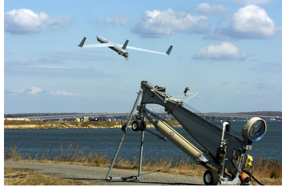
A ScanEagle unmanned aircraft is launched from a test range in Dahlgren, Va.
